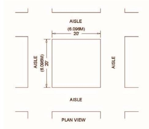
Overhead signs are permitted for Island Booths 20ft (6.09m) x 20ft (6.09m) or larger. Height limitation from the floor to the bottom of the sign is 20ft (6.09m) and must be directly over contracted space only.
